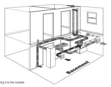
For this type of installation, it is not necessary for the forced-air blower to run while the unit is in operation. The 120 Hybrid is powerful enough to circulate fresh air to all rooms of the house without blower assistance.
