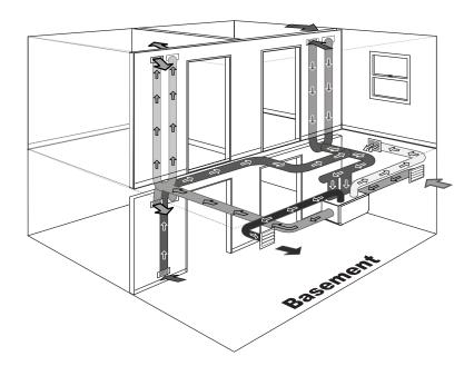
In the basement it is recommended to have at least one exhaust vent close to the floor as the humidity in a basement tends to concentrate near the floor.
