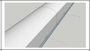
A cover plate can be used to close the gap between both halves if necessary. Using aluminum tape or duct tape seal the seam in the back where the two halves join together.
