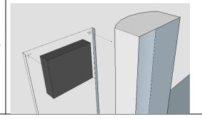
Before mounting the unit's back plate to the wall, attach the flex pipe to the collar on the back of the unit and insert the other end of the flex pipe inside the hole in the wall.(A 24" cable tie or a few small 9/16" screws can be used to affix the flex to the collar)
