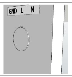
An electrical fitting needs to be installed. With the fitting installed the wire can be inserted inside the unit and connected.
