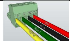
Now that the connector has been wired, insert it into the booster fan unit.
