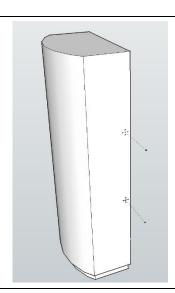
Separate the front aluminum piece (Front Cover) from the back galvanized piece (Back Plate).
