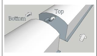
Secure the two halves together using ½" metal fastening screws.
